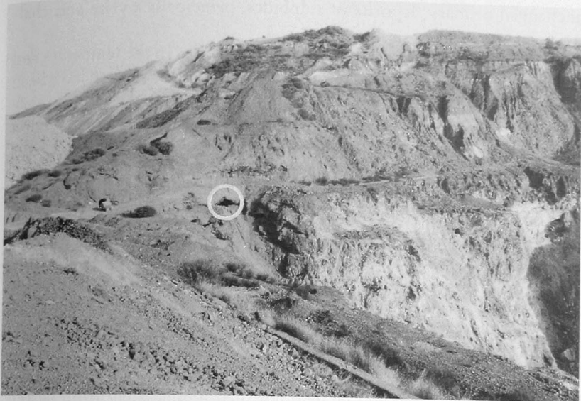
FIGURE 2.2 Corta Lago opencast mine at Rio Tinto, Huelva, Spain, showing the massive red weathered gossan deposits sat on the primary sulphidic ore body. The rich jarosite silver ore was found at the junction and the ancient workings are concentrated at this level. Note the small gallery, which leads to a complex system of workings (indicated).
