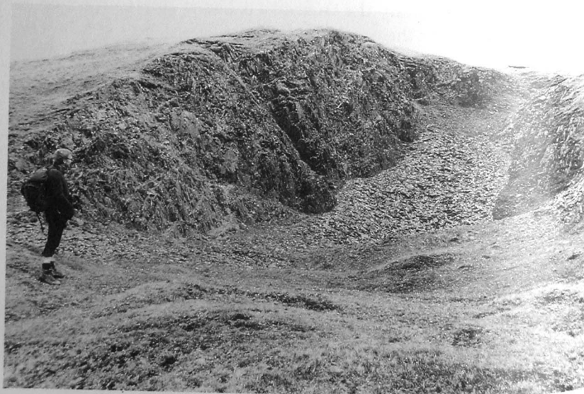
FIGURE 2.23 Bronze Age copper mine at Copa Hill, Cwmystwyth. Because of the width of the lode the mine developed as an opencast.
