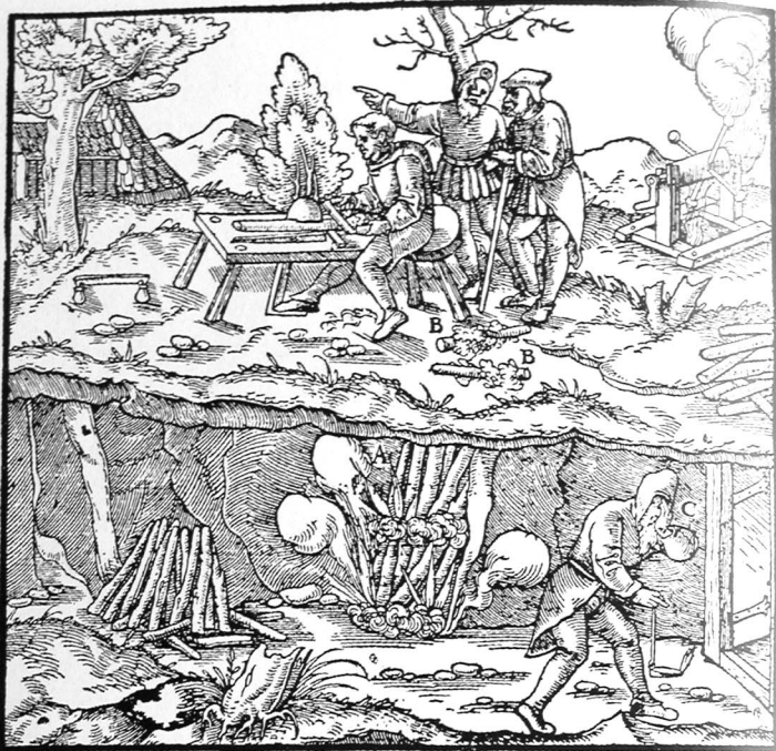
A—KINDLED LOGS. B—STICKS SHAVED DOWN FAN-SHAPED. C—TUNNEL.
