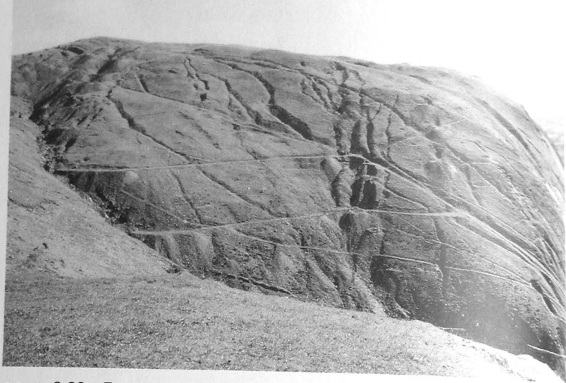
FIGURE 2.22 Four thousand years of mining history at Copa hill, Cwmystwyth. Note the series of channels directing water from the dam (Figure 2.49) to remove the glacial debris covering Comet Lode (running vertically down the hillside). The Bronze Age workings are at the very top of Comet Lode.
