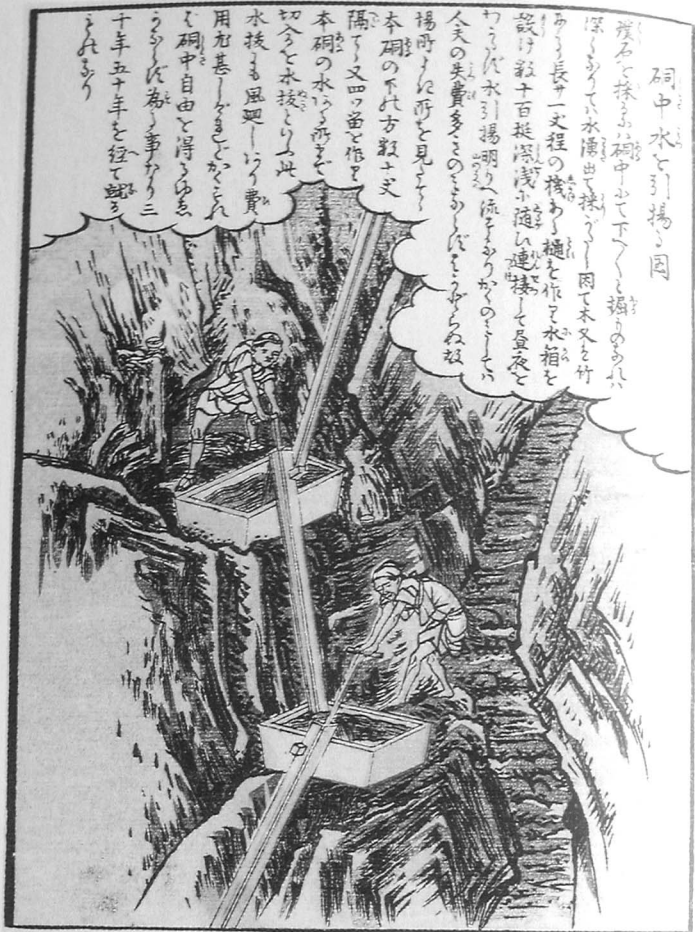
FIGURE 2.42 Nineteenth century Japanese system for raising water from mines using a series of hand pumps.
