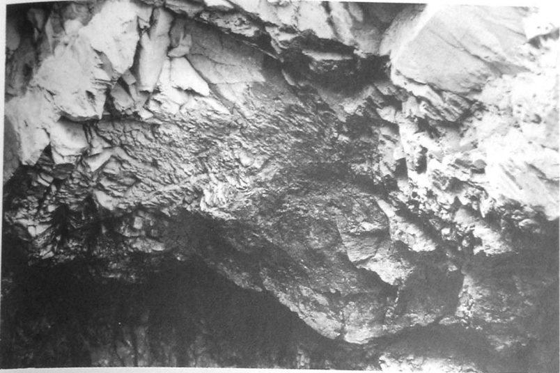
FIGURE 2.24 Well preserved batter marks made by stone hammers in the roof of a small gallery in the main opencast at Cwmystwyth. (The width of the rock shown is about 50 cm.)
