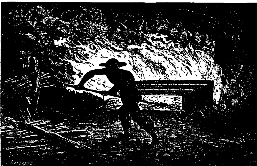
Figure 6 Miners at Rammelsberg in the Harz Mountains, Germany, directing the fires using an iron hood (from Simonin 1868 [21]).
