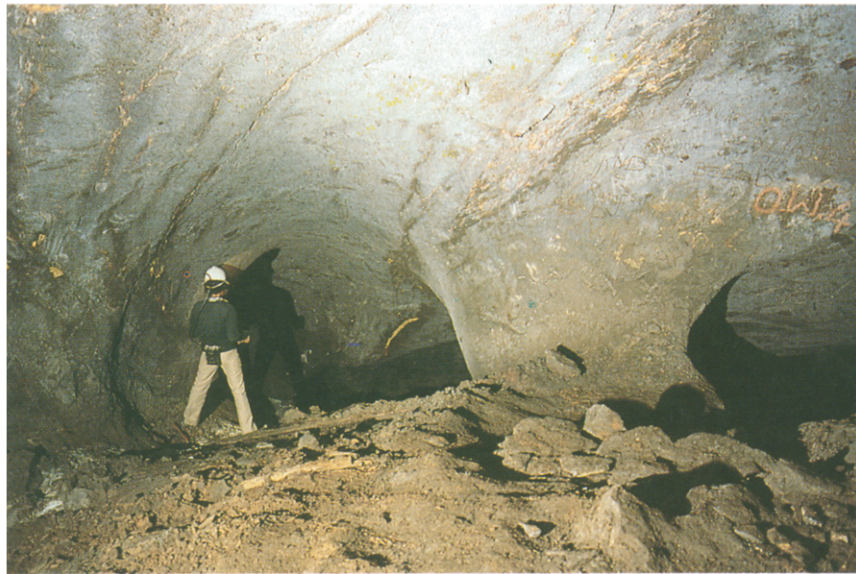
Figure 2 Large gallery mined by firesetting in the lead/zinc mines at Zawar, in the Aravalli Hills, Rajasthan, India, (late 1st millennium B.C.).
