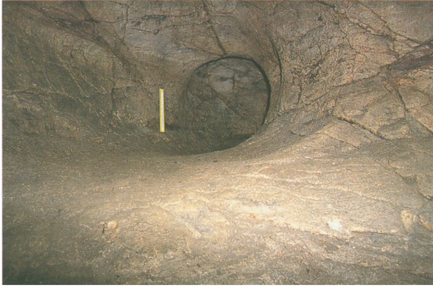
Figure 1 Smooth continuous walls are typical of fireset mine workings. These are in the tin mine at Kestel in the Taurus Mountains of Turkey, and date from the third millennium B.C. (30 cm scale).
