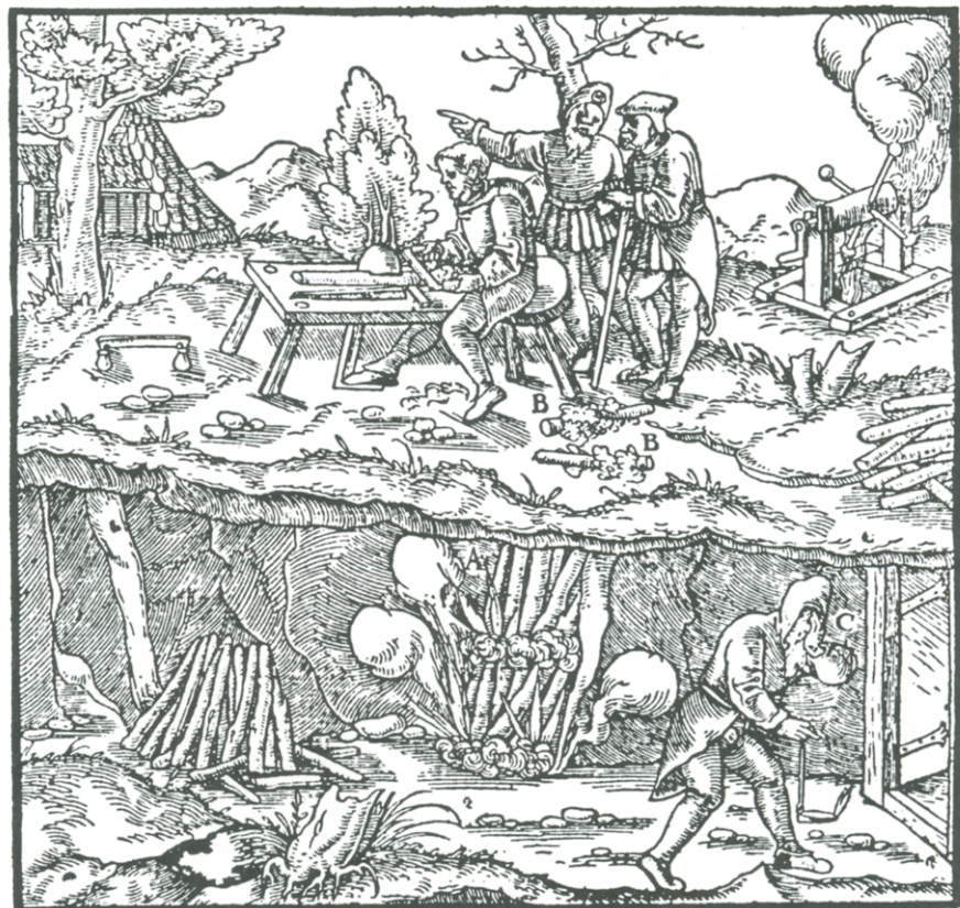
A—KINDLED LOGS. B—STICKS SHAVED DOWN FAN-SHAPED. C—TUNNEL.
