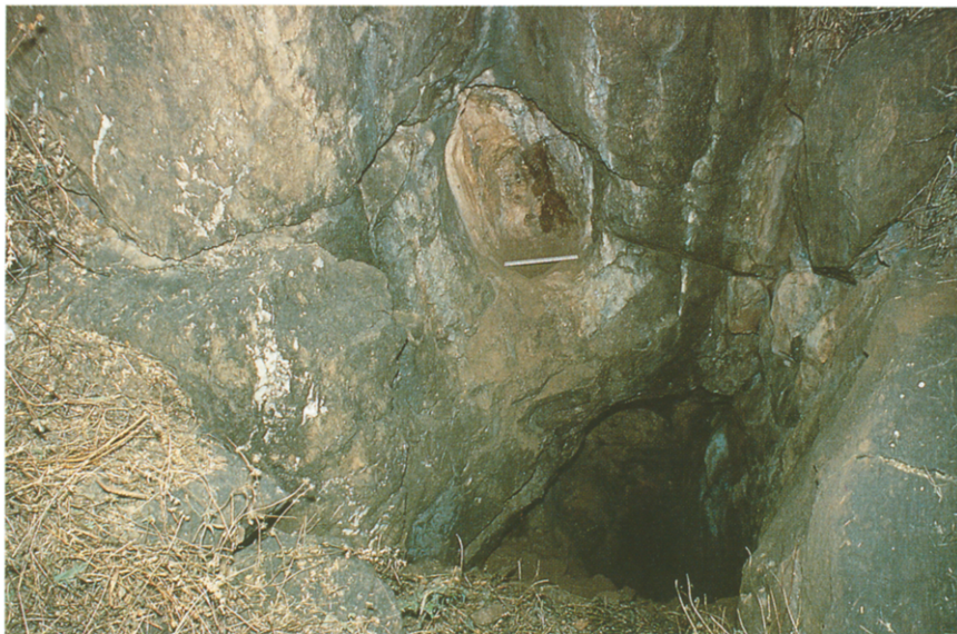
Figure 7 Vertical shaft sunk by firesetting at Zawar. Note the small fireset working on the far side of the shaft.
