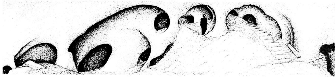
Fig. 2 : Zawar Mala Mine in India showing upper, earlier period working and lower, later period retreat working with steps leading towards the Upper Chamber, 260° panorama (CRADDOCK, 1994 : fig. 4).
